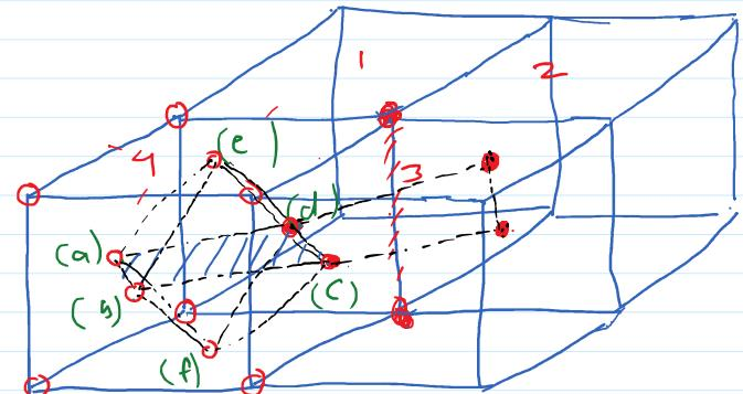
ii) On joining these faces, an octahedron is generated. Thus this unit cell has one octahedral void at the body centre of the cube.
